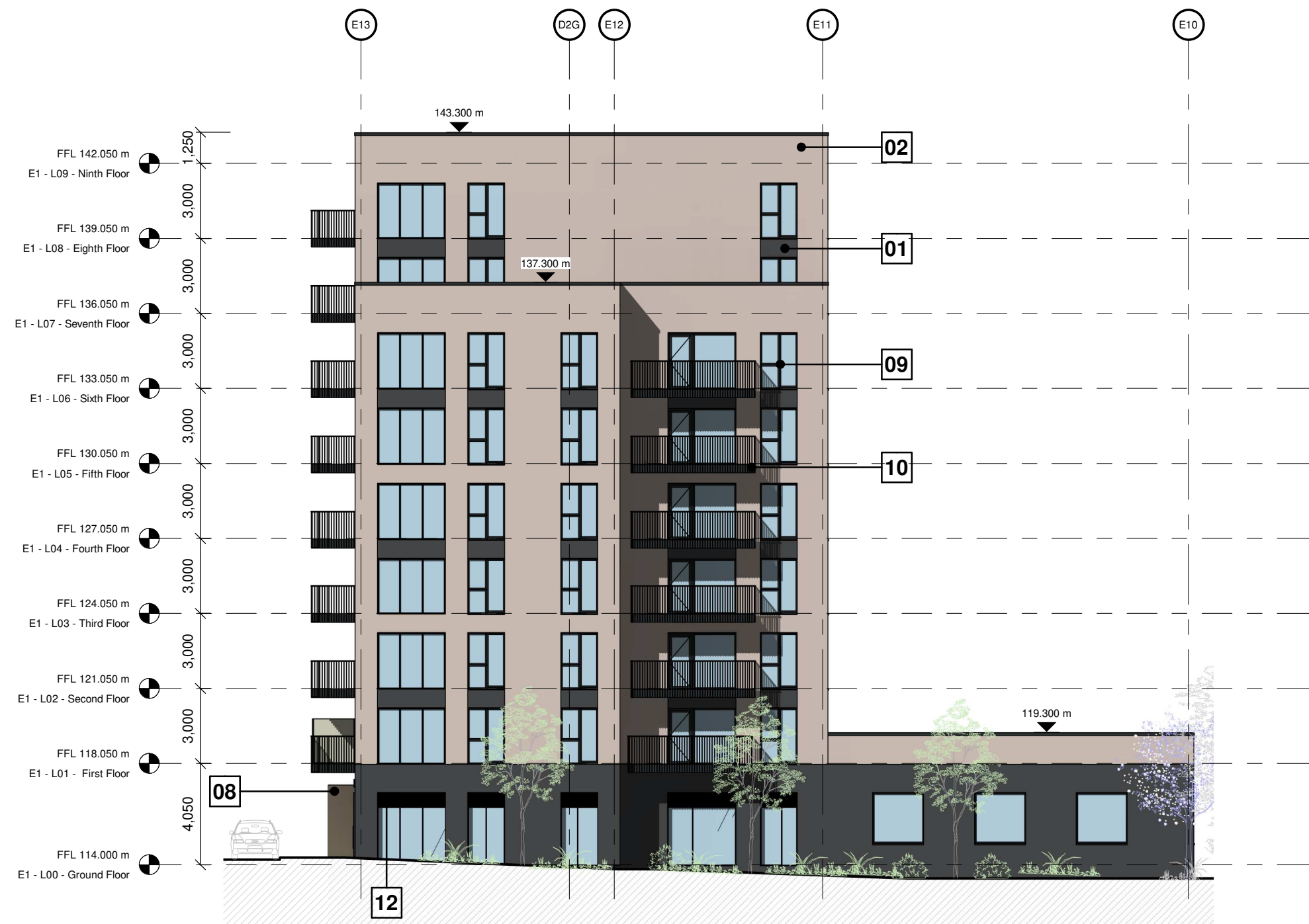
3 PROPOSED ELEVATION - BLOCK E1 - EAST 1 : 200
