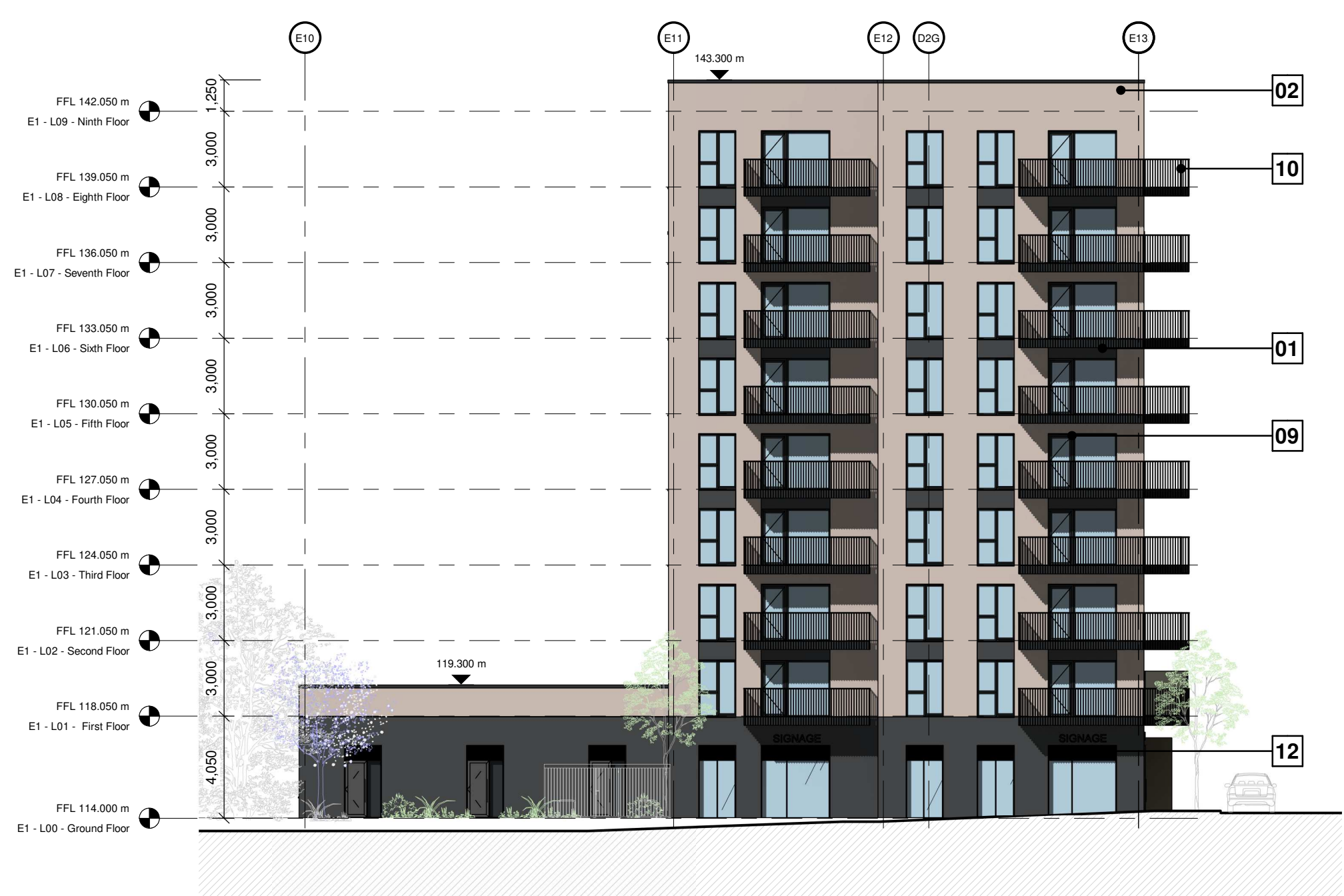
2 PROPOSED ELEVATION - BLOCK E1 - WEST 1 : 200
